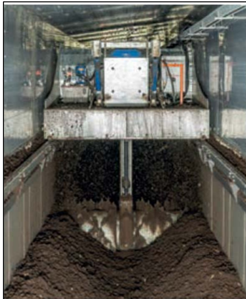
Figure 8: Inside the composting unit - container lined with stainless steel
